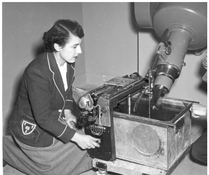
Sylvia performing depth dose measurements on the Cobalt-60 unit. Sylvia notes the snappy dress of the time.
