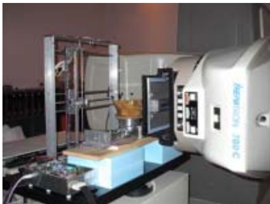
The T780C Cobalt-60 unit in the KRCC tomotherapy benchtop configuration when not treating emergency patients.
