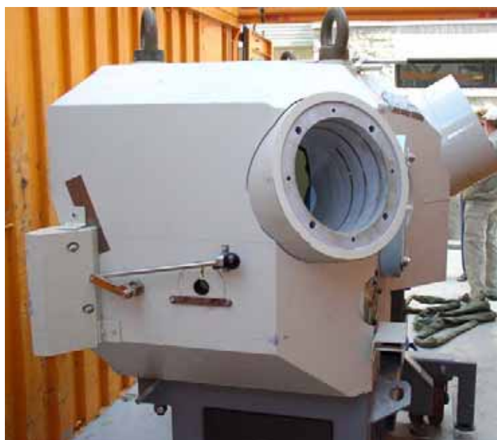
Figure 4: Image of the loading cell that mates the ball head with the shipping flask for cobalt source transfers.
