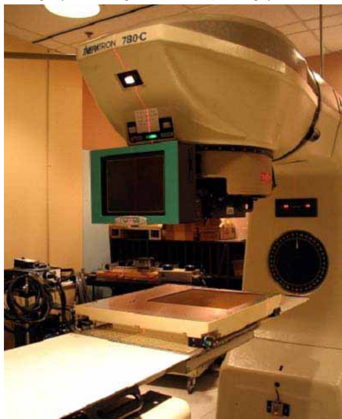
The world's first MIMIC equipped Co-60 unit with a Varian SLIC portal imager for Co60CT (not mounted in picture).
