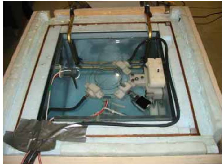
Figure 2: Photograph of the ESW calorimeter taken from above with the lid removed.
