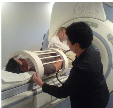
Figure 1: Volunteer being scanned for a hyperpolarized ^3\text{He} study on the 3 T. The RF coil around the volunteer transmits and receives at the ^3\text{He} Larmor frequency (97.3 MHz at 3 T).
