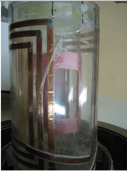
Figure 4: Home-built ^3\text{He} RF coil for rat imaging with the 0.075 T scanner. The outer coil is for uniform RF transmission, while the smaller, inner coil is for sensitive RF reception.
