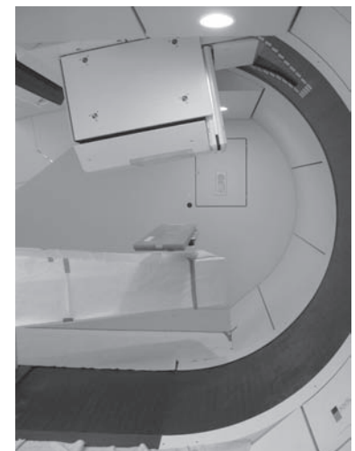
Figure 3: Newest gantry at PSI designed for fast scanning and includes in-room CT guidance.
