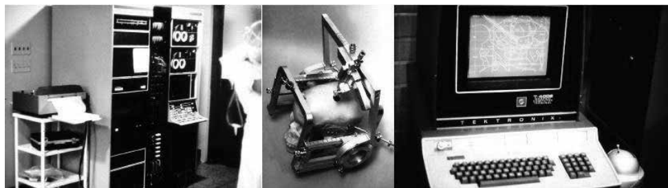
The PDP-12 computer parked outside the operating room, stereotaxic frame with thalamic recording probe on a skull as it would be positioned on a real patient, and the Tektronix storage-screen computer terminal used to show the probe tip location on a digitized brain atlas, scaled to the correct size, during surgery for Parkinson’s disease. (1971)
